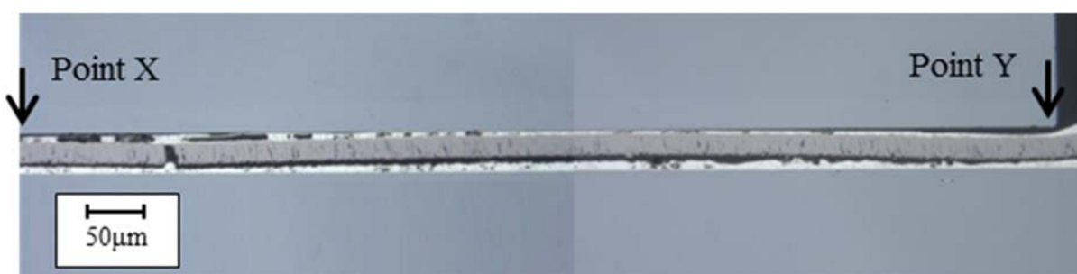
図 2-18 Optical microscope photograph of the X-Y cross-section in SAT image for specimen #2( R=22.7 \times 10^{-6} \text{m}^2\text{K/W} ).
