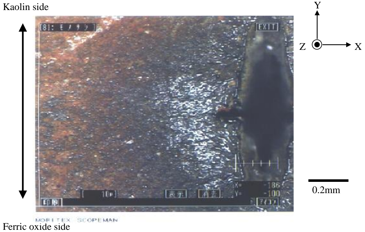
Fig.3.9 Photograph of the laser processed functionally graded material. 50%-50%layer, laser fluence: 1.0 kJ/cm 2 , repetition frequency: 10Hz, number of pulse: 400.
